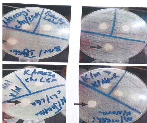
Fig. 2. Agar plates showing zones of inhibition of antimicrobial residue using Bacillus subtilis .
